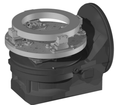
Clamping Device: 2x VC-74 Fixture: Perforated grid plate
